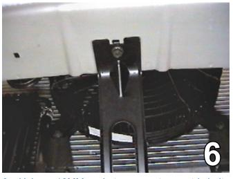
Using a 10MM socket, remove two metric bolts from just below the metal bumper, from the center bumper support. Set the metric bolts and bumper support aside to be reinstalled later.
