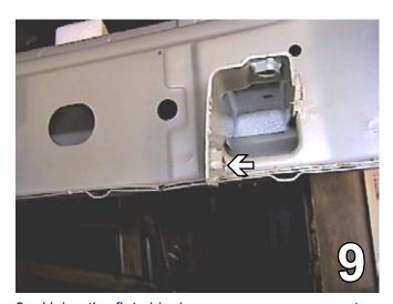
Using the flat chisel, remove one square nut from the bumper bracket. Do this to both sides of the vehicle.
