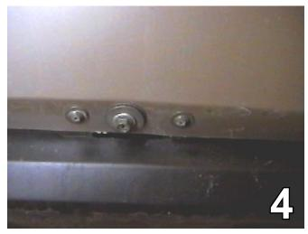
4. Using a 10MM socket remove three metric bolts and for Phillips head screws on the bottom edge of the fascia. **2004 Models Only.**
