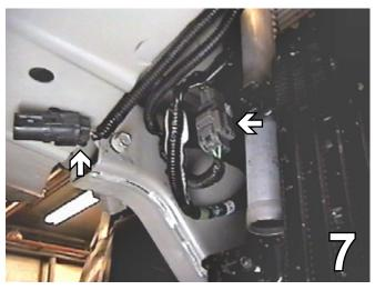
Disconnect the electrical sensor from the metal bumper and wiring harness from the frame. Tie the harness and sensor up away from the frame area.
