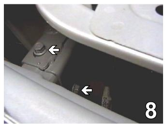
8. Using a 12MM socket, remove two metric bolts from the top and lower frame end. Do this to both sides of the vehicle. Pull metal bumper forward to remove. Set metric bolts and metal bumper aside to be reinstalled later.
