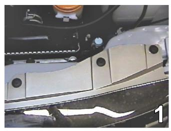
Remove six pushpins from the top edge of the grille between the headlight assemblies.
