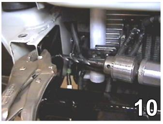
10. Using the vise grip, clamp the baseplate to the frame, align the lower front hole of the baseplate with existing hole for the bumper bolt. This should allow baseplate to extend 1/8" forward of the frame end while maintaining a level position. Using the baseplate as a template, drill all holes into the frame with the 13/32" drill bit. Do this to both sides of the vehicle.
