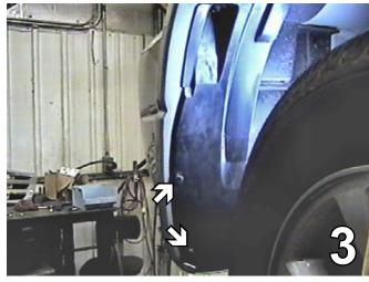
Using a 10MM socket, remove one metric bolt and two pushpins from just forward of the front tires. Do this to both sides of the vehicle. Set metric bolts and pushpins aside to be reinstalled later.
