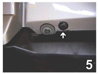
5. Remove two pushpins from the fascia's lower edge, 2004 Models Only. Pull the fascia forward, disconnect the electrical lines on the fog lights and set aside to be reinstalled later. Set the pushpins aside to be reinstalled later.
