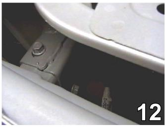
Install the metal bumper to its original position and tighten the two top bolts with the 12MM socket. Please refer to the LOCTITE note to the left.
