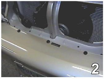
2. Remove three pushpins from the fascia just below the grille area. 2005 Models: will have seven pushpins to remove.
